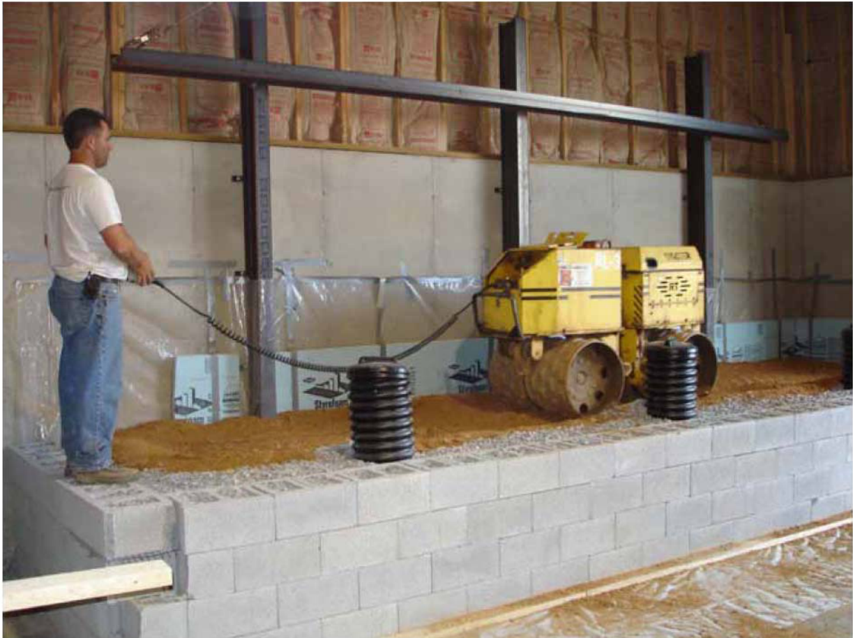
Picture shows the full-scale test wall constructed at Sleeve-It Facilities. Two Sleeve-It 1224R Systems are visible in the foreground. A steel reaction frame used as part of the loading system is visible in the background.
