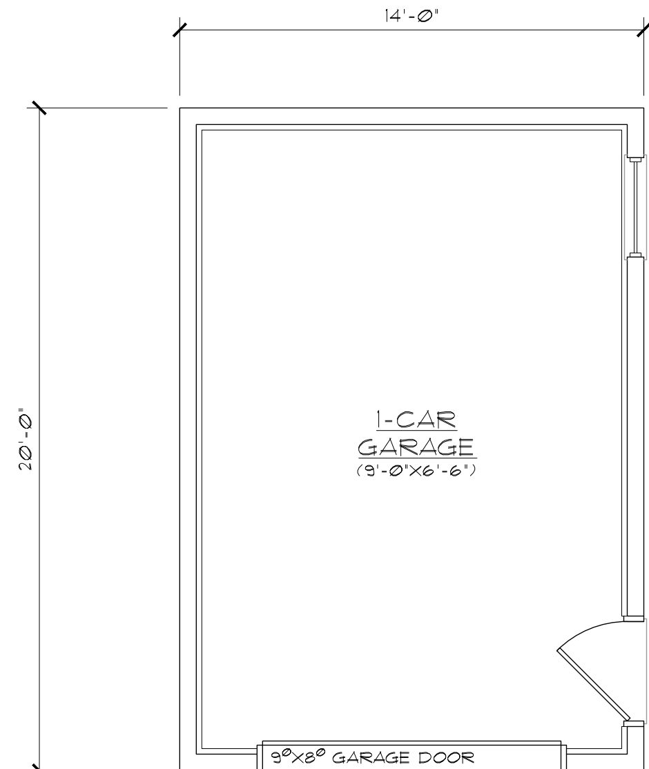
3 PROPOSED GARAGE PLAN (280 S.F.) SCALE: 1/4" = 1'-0"
