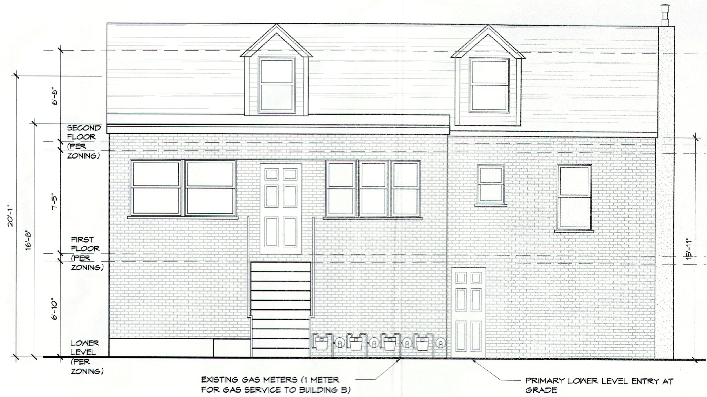
20 BUILDING 'A' FRONT (EAST) ELEVATION SCALE: 1/4" = 1'-0"
