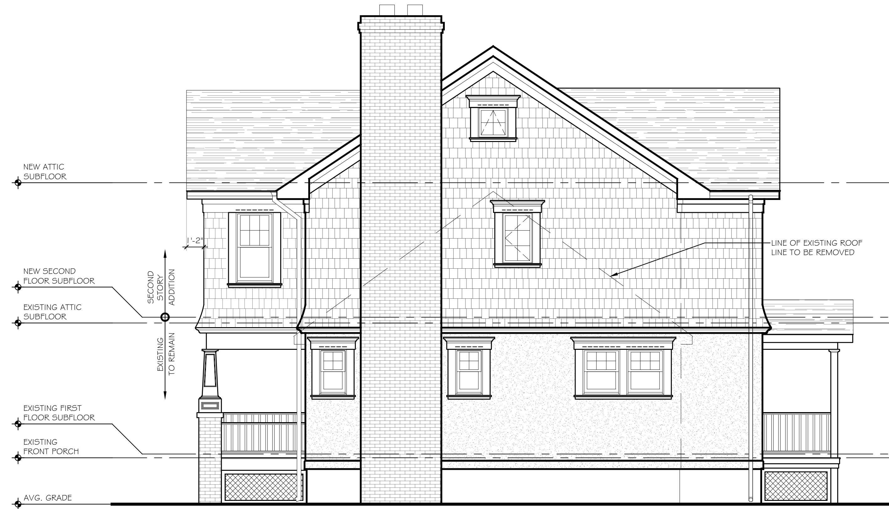
2 RIGHT SIDE ELEVATION SCALE: 1/4" = 1'-0"
