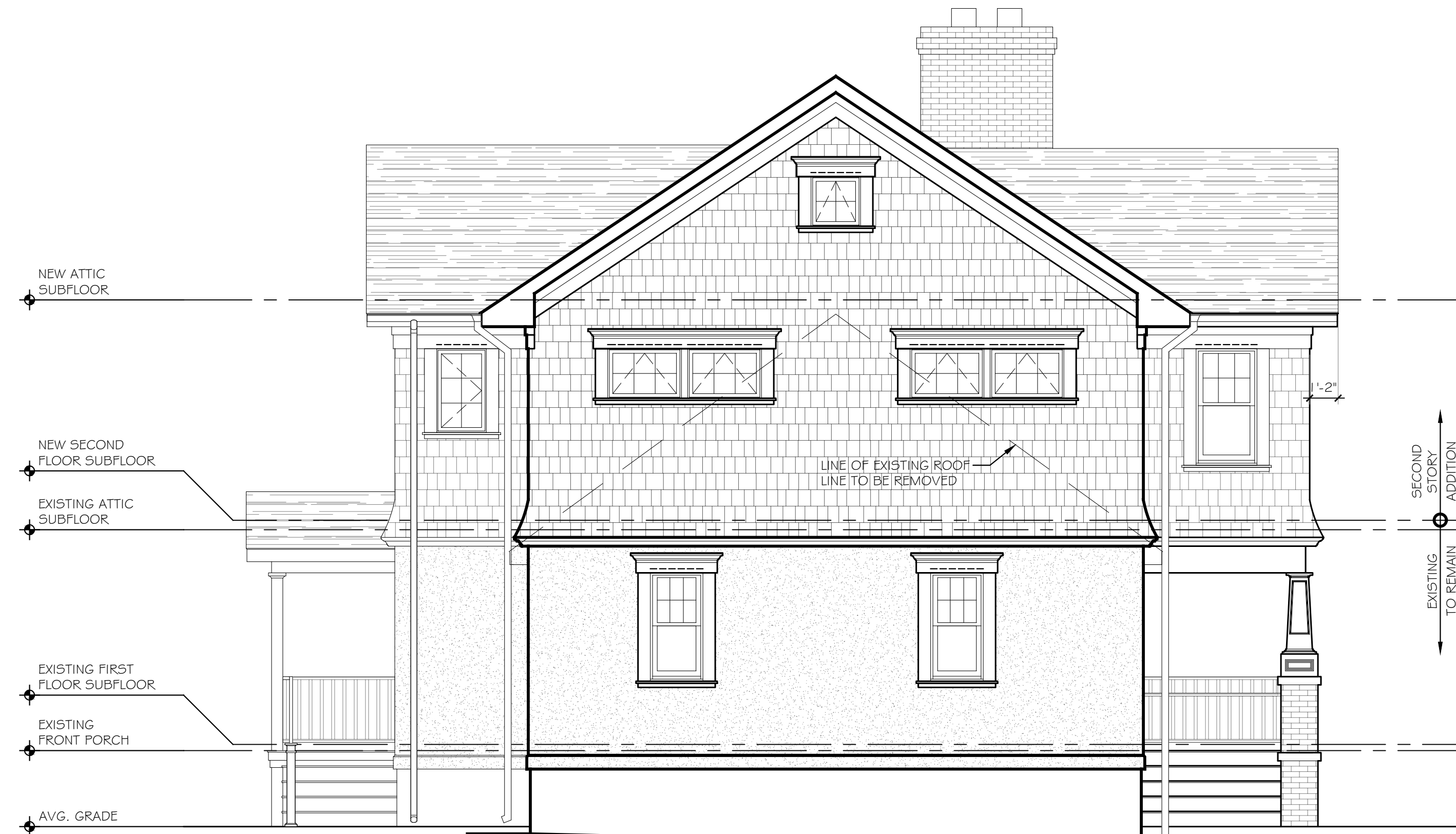
4 LEFT SIDE ELEVATION SCALE: 1/4" = 1'-0"
