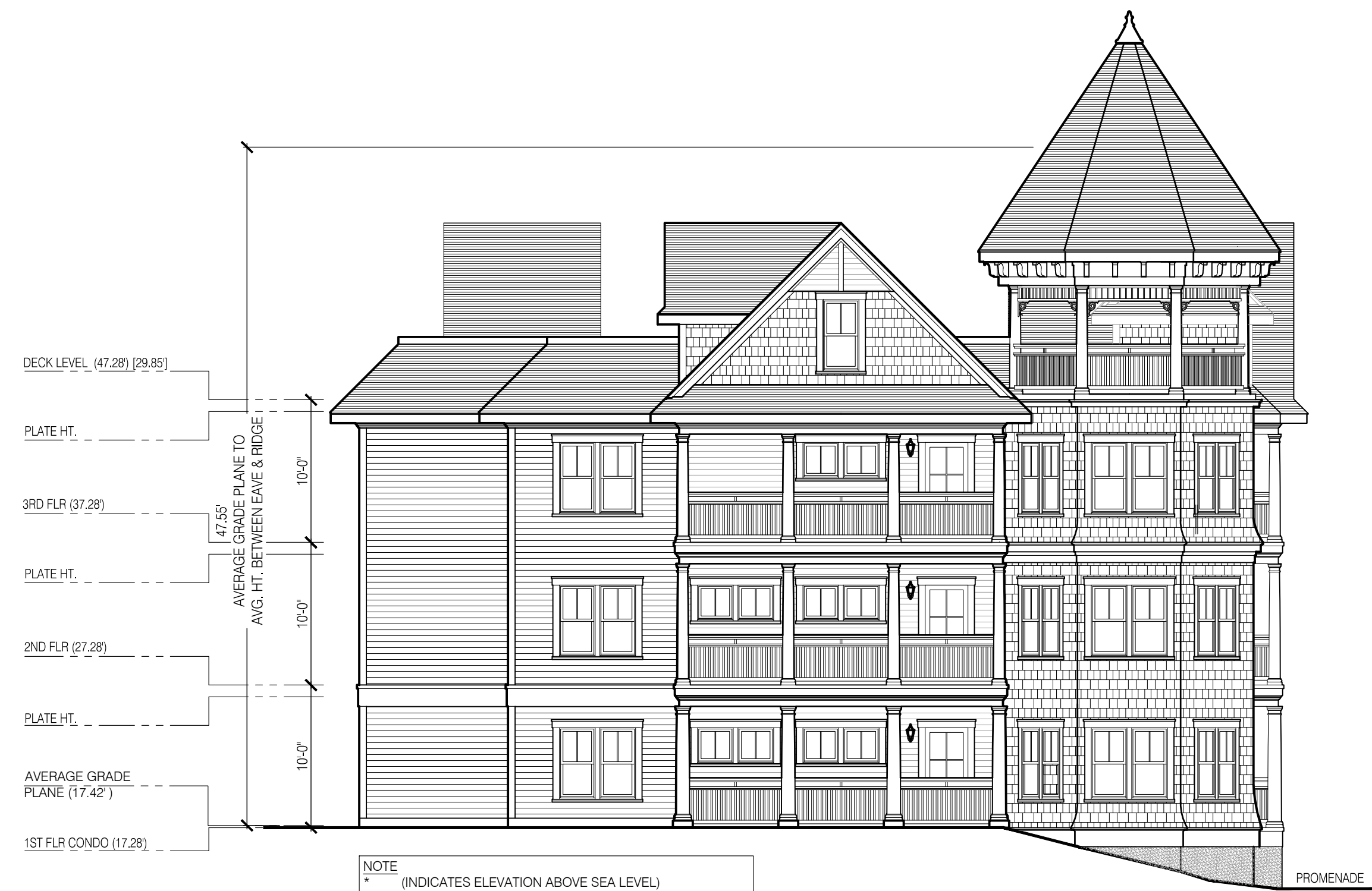
② BUILDING 2 - EAST ELEVATION 1/8" = 1'-0"
