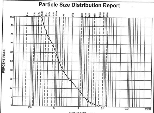
GRAIN SIZE - mm. % Sand % +3" % Fines % Gravel Coarse Fine Silt Clay 0.0 72.1 21.0 6.0 0.9
