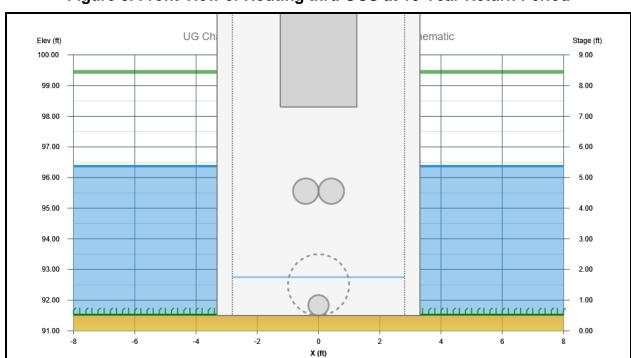
Figure 8. Front View of Routing thru OCS at 10-Year Return Period
