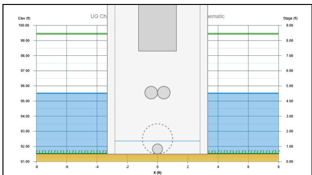
Figure 6. Front View of Routing thru OCS at 2-Year Return Period
