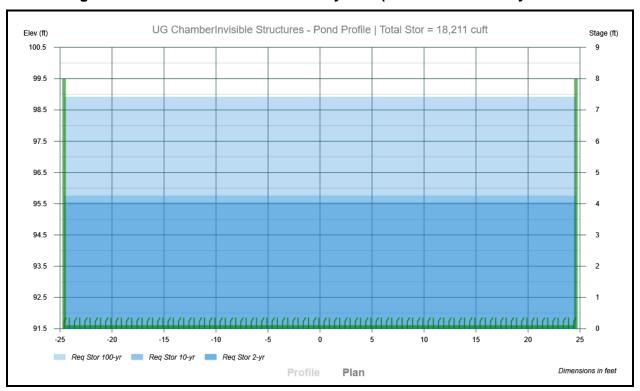
The system will be located 0.25' (3") below the inflow from the Kraken Manufactured Treatment Device. The 8.00' foot depth is designed to minimize cover on the system to 3.0 feet maximum per manufacturer instructions. The bottom of the system will be located at elevation 91.50 which is 3.5 feet above the mottling discovered in Test Pit #19 which is shown in the figures below.
