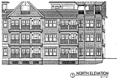
Illustration F.1.b. — North elevation of Condominium Building One showing proposed clapboard reveal at first floor (wide) and upper floors (narrow) (Sheet A-6).
