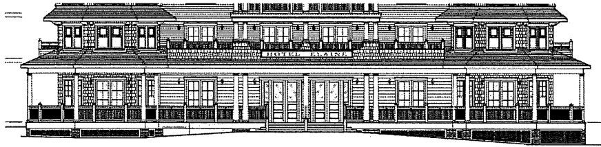
Illustration E.3.a. — First-floor, south elevation of the Hotel showing inappropriate Colonial Revival windows (Sheet A-11).
