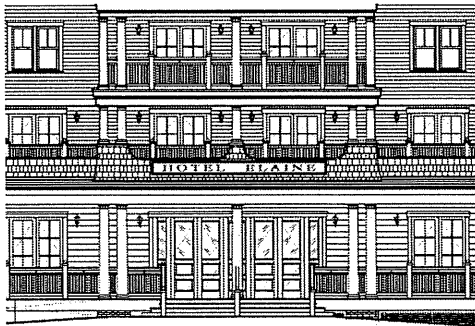
Illustration D.2. — The south elevation (Sheet A-11) showing proposed double set of double ½ doors, with non-conforming single side-light windows to the left and right.
