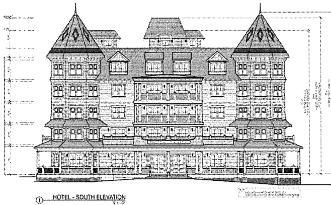
Illustration C.3. — South elevation of the Hotel showing proposed diamonds and banding on tower roofs (Sheet A-11).
