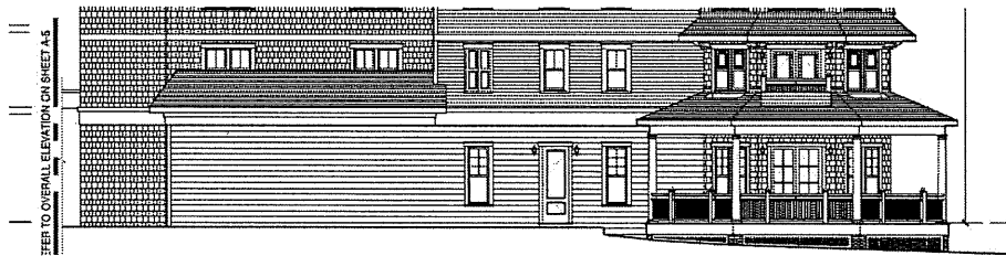
Illustration E.3.b. — First floor, west elevation of the Hotel showing inappropriate Colonial Revival windows (Sheet A-12).
