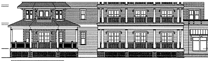
Illustration E.3.c. — First floor, east elevation of the Hotel showing inappropriate Colonial Revival windows (Sheet A-12).
