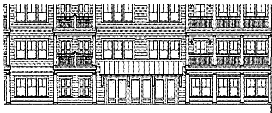
Illustration C.13. — South elevation of Condominium Building One showing proposed standing seam roof over main building entrance (Sheet A-6).
