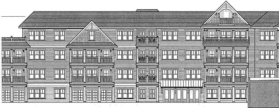
Illustration E.8.b. — Detail of south elevation of Condominium Building Two showing stacked courses of double and triple windows in non-historic fenestration patterns.
