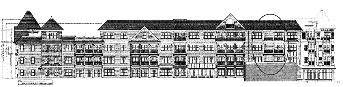
Illustration I.10. — South elevation of Condominium Building One showing balconies with no lighting indicated.
