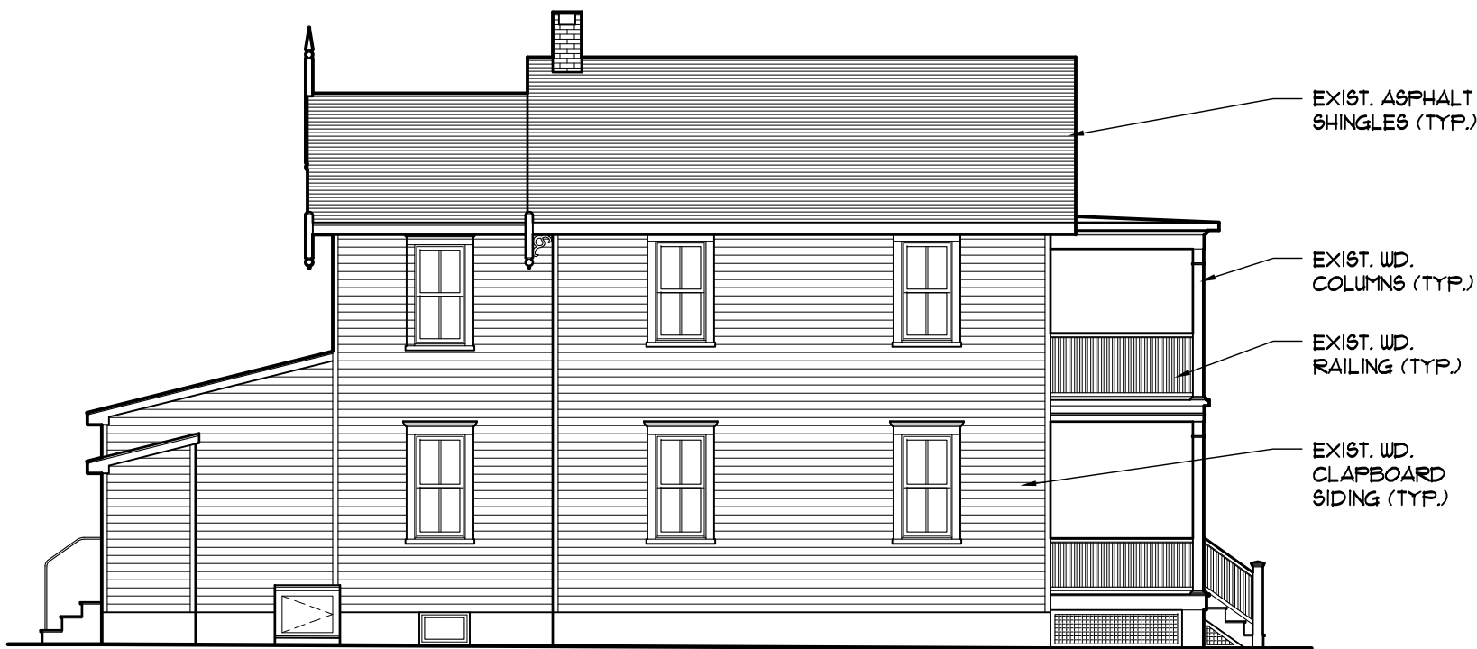
EXISTING SIDE (EAST) ELEVATION 1/8" = 1'-0"
