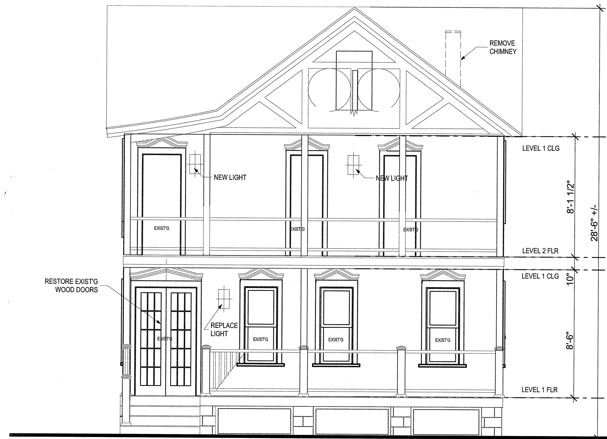
Front Elevation (North)
