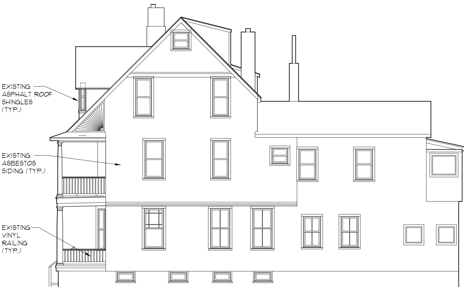
EXISTING SIDE (EAST) ELEVATION 1/8" = 1'-0"
