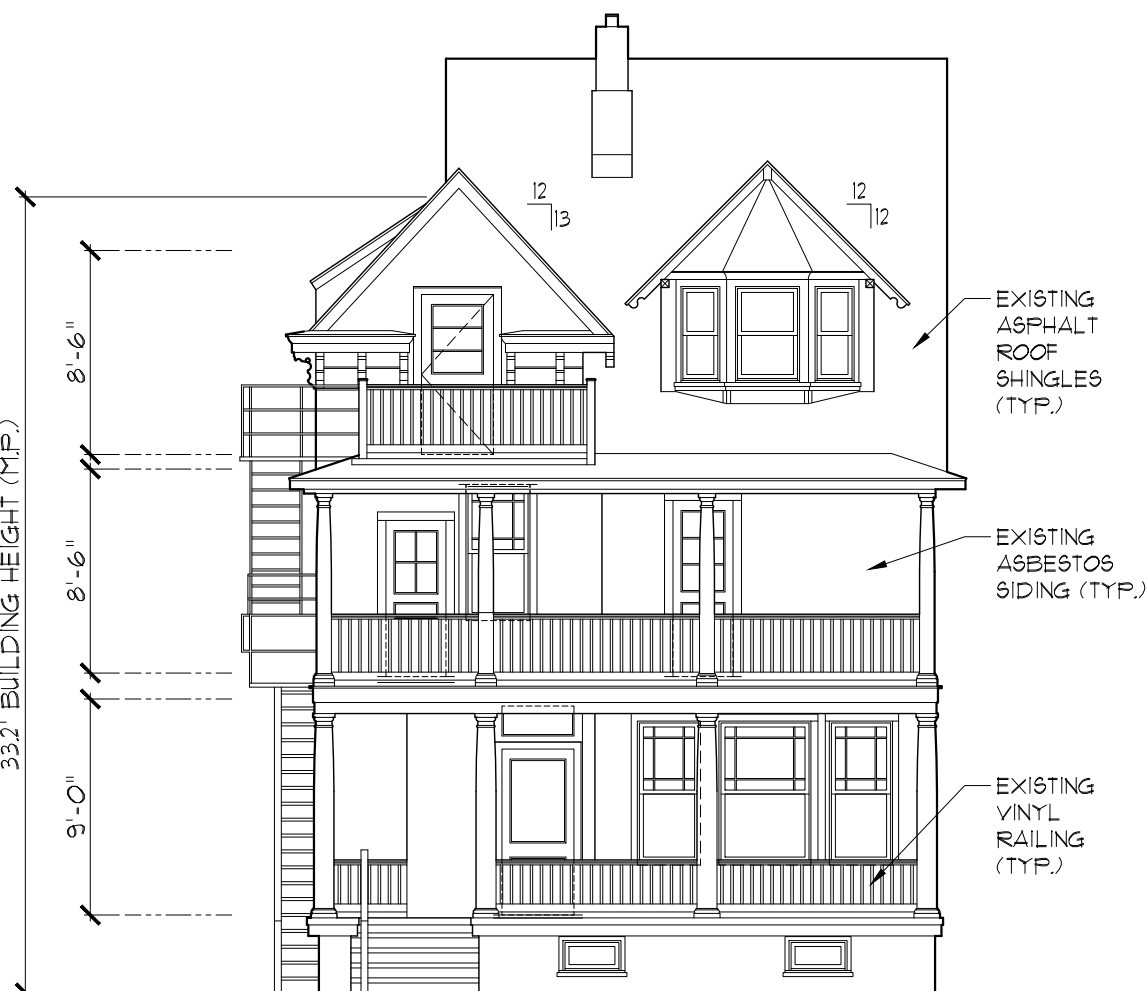
EXISTING FRONT ELEVATION 1/8" = 1'-0"
