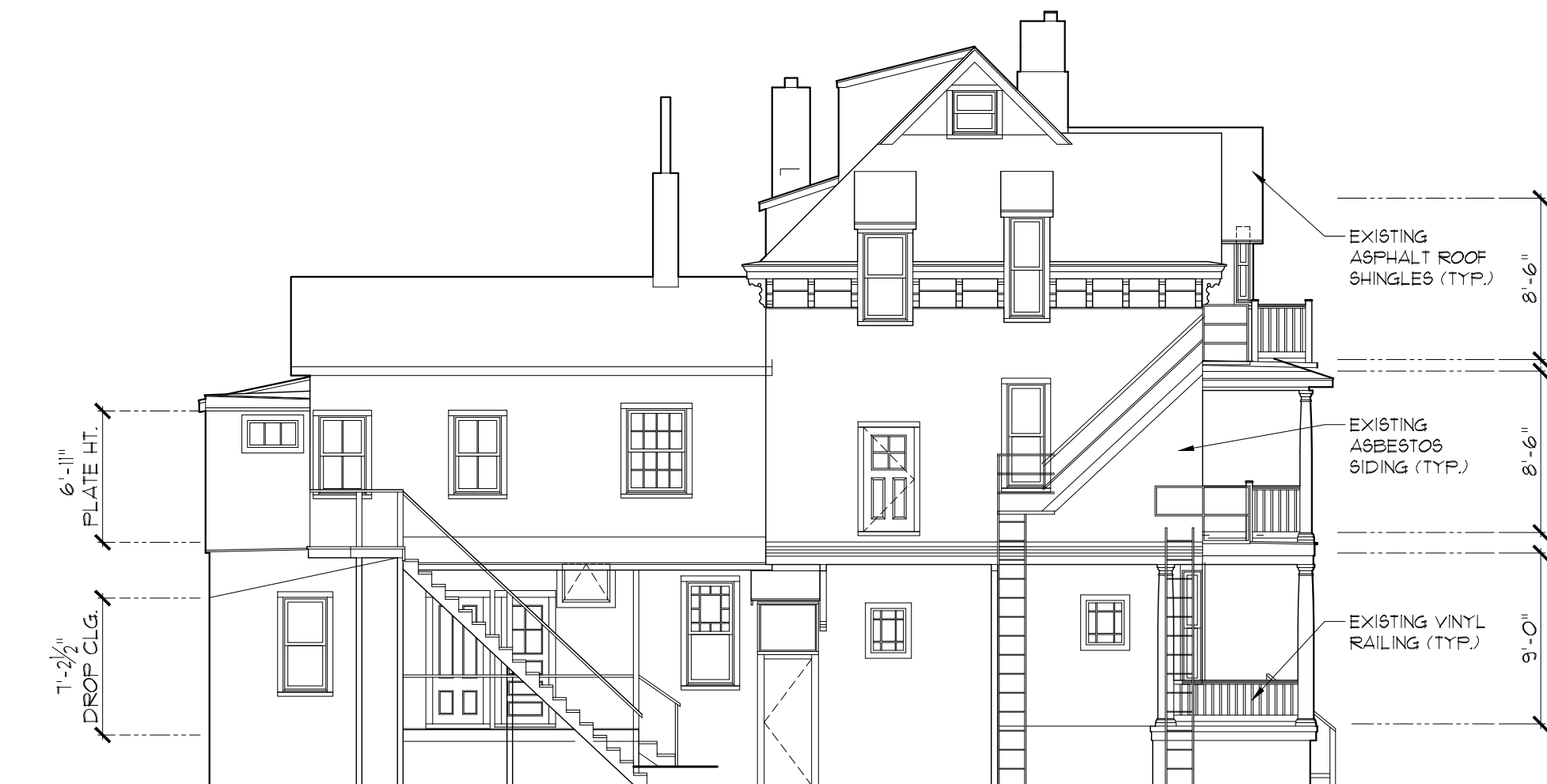
EXISTING SIDE (WEST) ELEVATION 1/8" = 1'-0"
