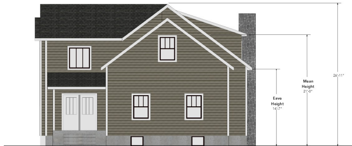
3 PROPOSED FRONT ELEVATION Scale: 3/16" = 1'-0"
