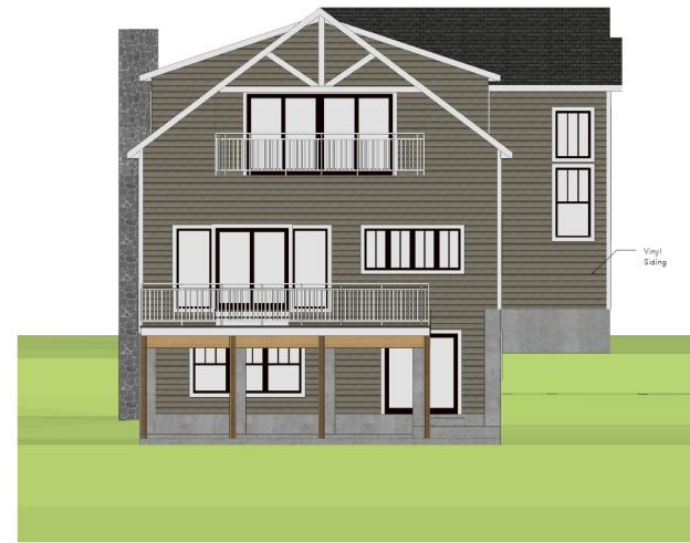
2 PROPOSED REAR ELEVATION Scale: 3/16" = 1'-0"
