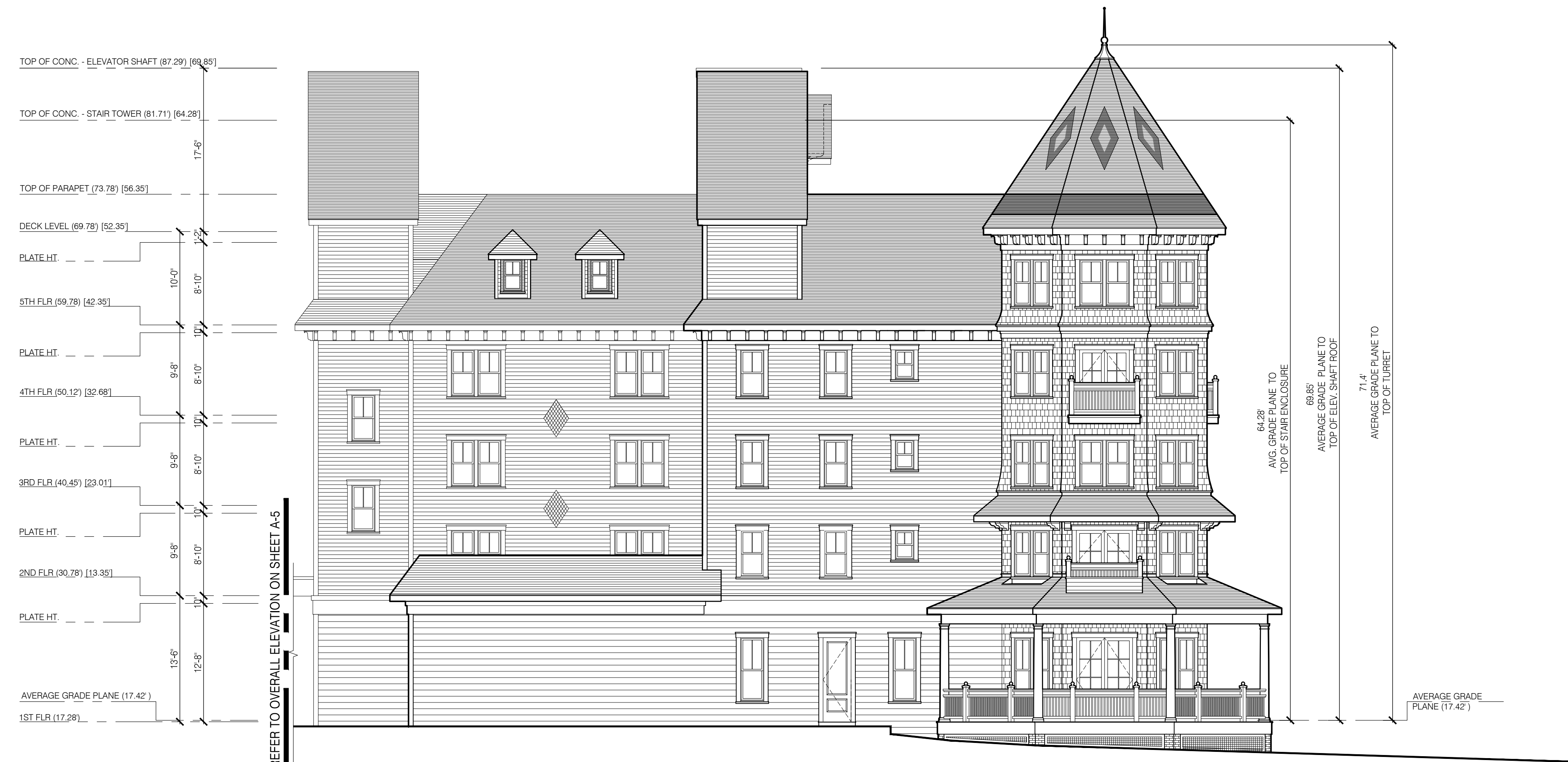
NOTE * (INDICATES ELEVATION ABOVE SEA LEVEL) (INDICATES ELEVATION ABOVE AVERAGE GRADE PLANE) ② HOTEL - WEST ELEVATION 1/8"=1'-0"
