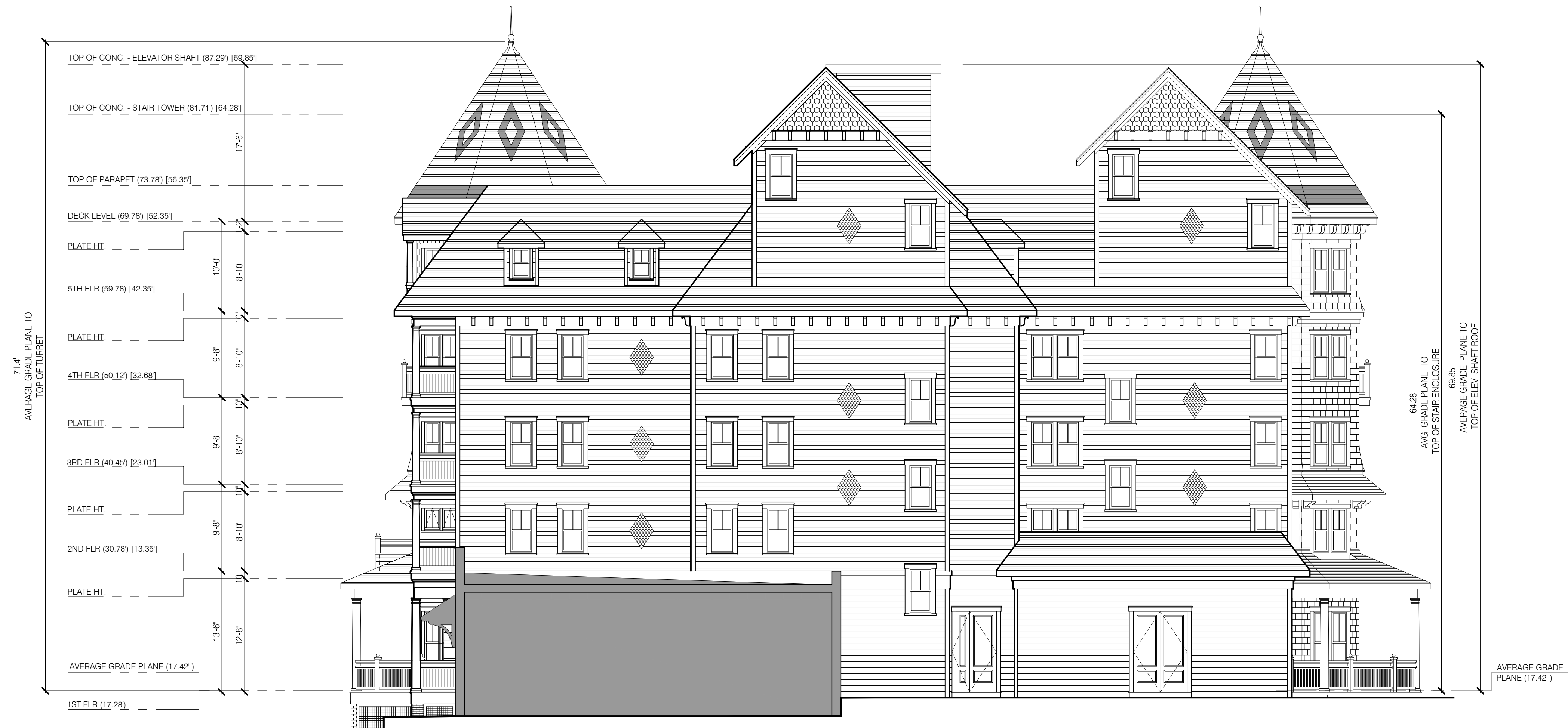
NOTE * (INDICATES ELEVATION ABOVE SEA LEVEL) (INDICATES ELEVATION ABOVE AVERAGE GRADE PLANE) ① HOTEL - NORTH ELEVATION 1/8"=1'-0"
