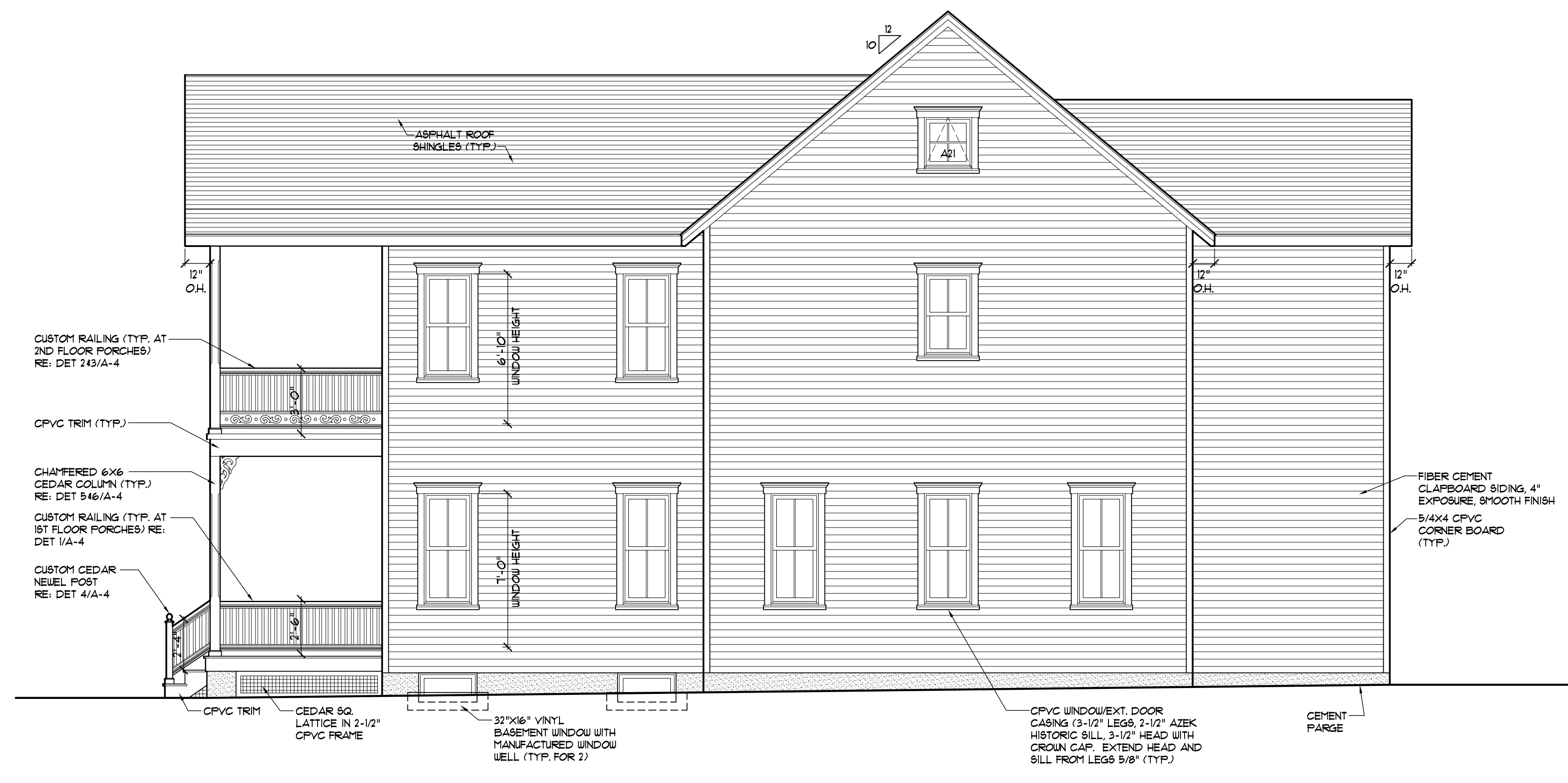
SIDE ELEVATION (WEST) 1/4" = 1'-0"
