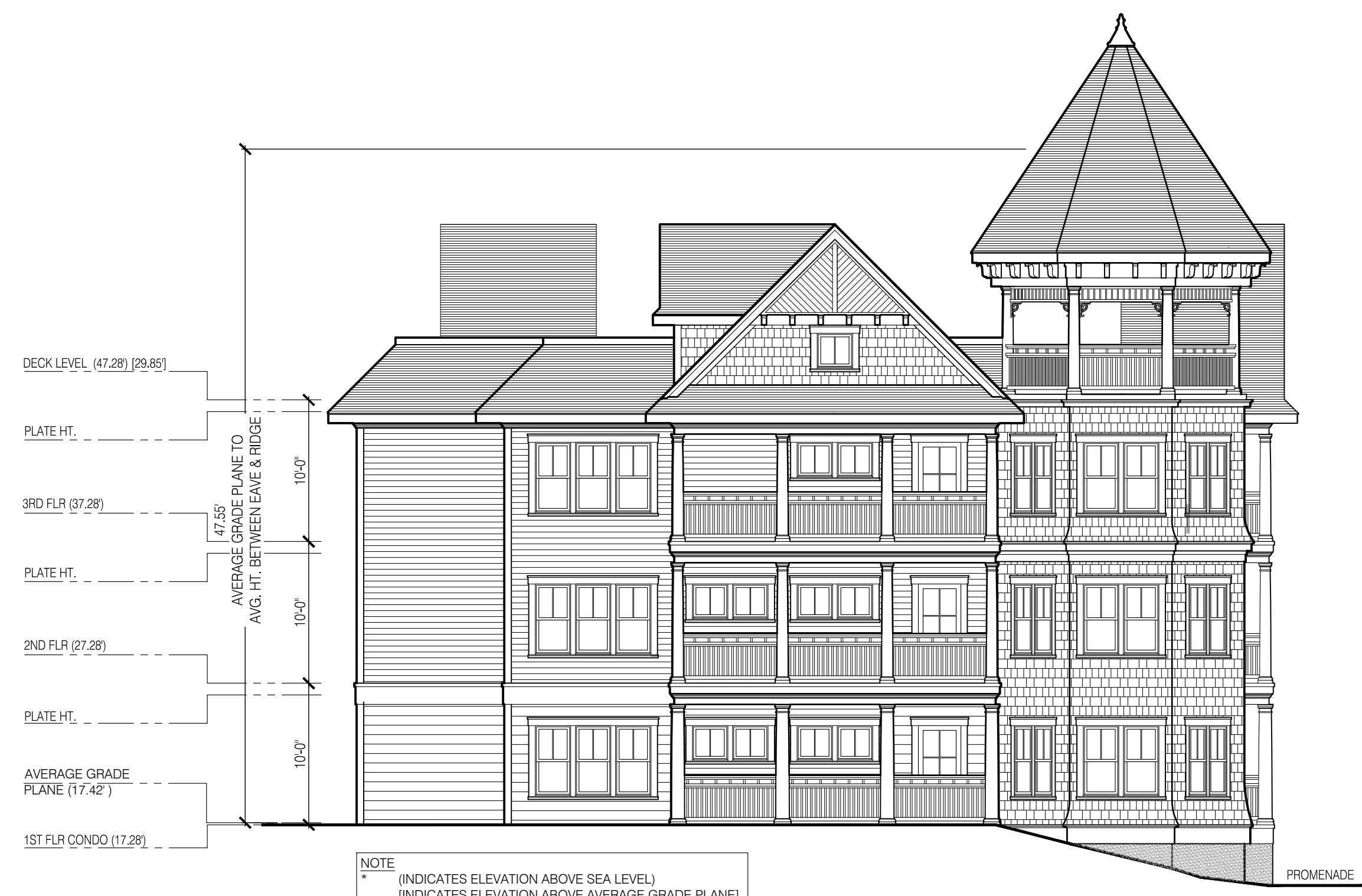
② BUILDING 2 - EAST ELEVATION 1/8" = 1'-0"
